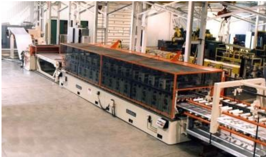
Figure 1: Inline Roll Former (Photo courtesy The Bradbury Co.)
