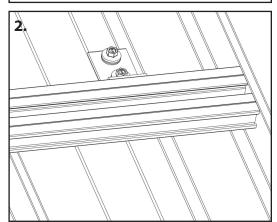
**3. Placing second strut on roof (do not fasten down yet):** Following the previous steps, place the second strut at the desired location. so that the bolt slots within the two GRIPPERFIX Struts are the same distance apart and consistent with the distance between mounting locations on the base of the object being mounted. (Fig. 3). DO NOT fasten to roof at this point.
