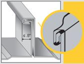
For horizontal seams under .5", crimp the seam to 180 degrees at desired clamp location.
