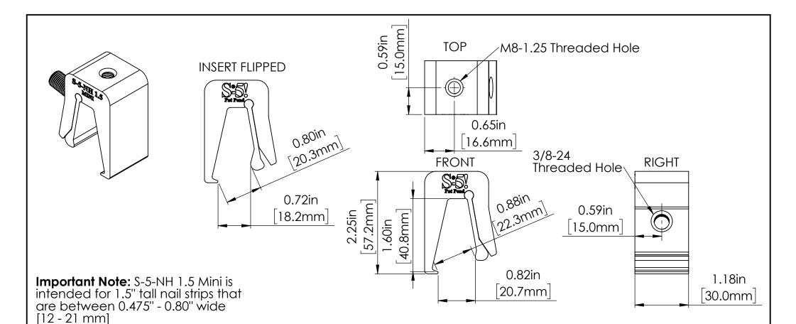
**Important Note:** Insert is intended to bend and the roof material is intended to compress when setscrew is torqued
